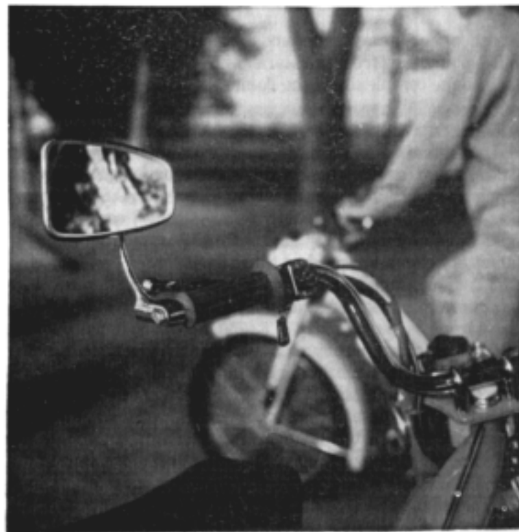
Fig. 1-1. A rearview mirror that meets the new regulations and folds for storage.
