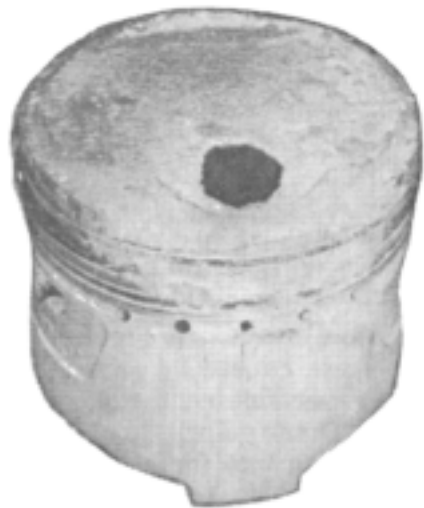
Fig. 2-14. Preignition does this to a piston. (Courtesy Champion Spark Plug Co.)
