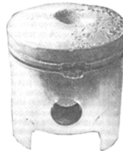
Fig. 2-16. Detonation makes short work of pistons. (Courtesy Champion Spark Plug Co.)
